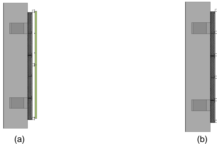
Fig. 4 – The concept of a modular facade with aerogel insulation and cladding of (a) composite panels (b) solar panels
