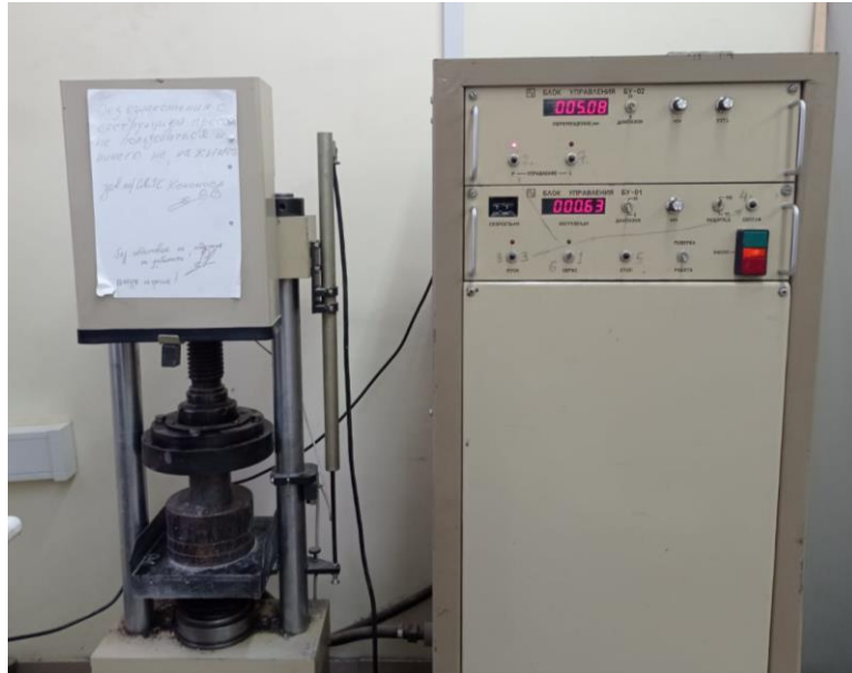
Fig.2 – Testing of samples for compressive strength and determination of the elastic modulus: upper indication – displacement, MPa; lower indication – force load, kN
