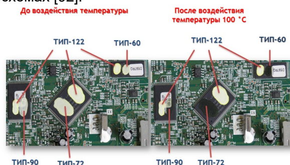
Fig.10. - Using a TYP melting temperature indicator in a microcircuit
