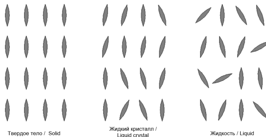
Fig. 4 - The difference in the order and orientation of molecules in solids, liquids and liquid crystals
