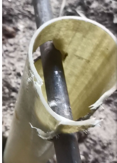
Fig. 4 – FRP delamination after oversized torque moment application Image by the author of the article
