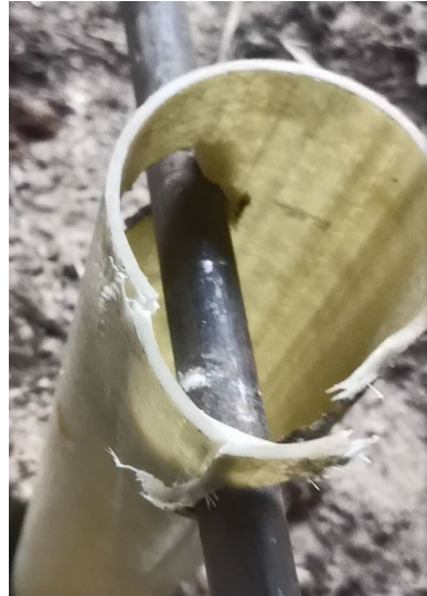
Fig. 4 – FRP delamination after oversized torque moment application.
