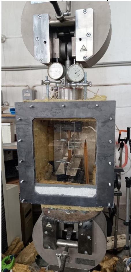
Fig. 1 – Thermostatic camera for cured polymer samples tensile testing
