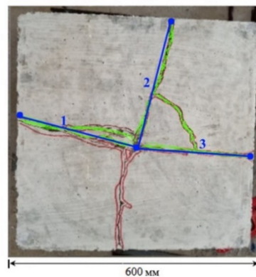
Fig. 7 - XRD analysis of samples: a) control composition, b) composition with 35% ASC : K_{сув} = l_f / l_s : 1 - (52 cm)/(34 cm) = 1.53; 2 - (58 cm)/(35 cm) = 1.66; 3 - (57 cm)/(34 cm) = 1.68
