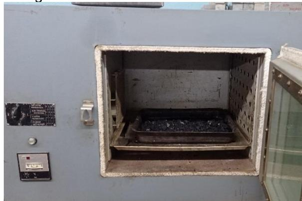
**Fig. 2 – Bitumen-limestone crushed stone on metal trays in ventilated thermal furnace**
