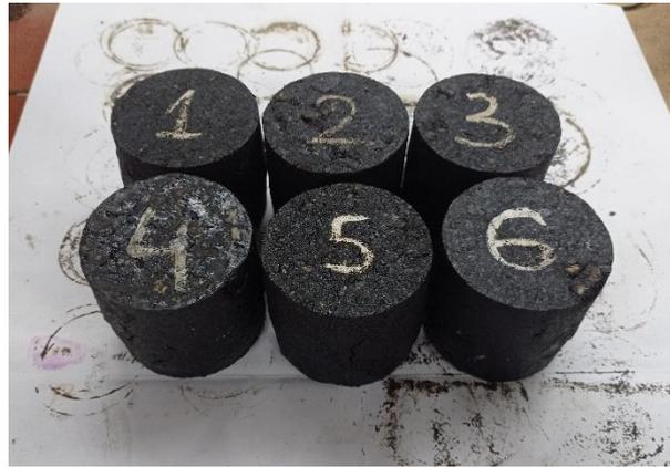
**Fig. 1 – Standard cylindrical specimens size of 71.4 mm**
