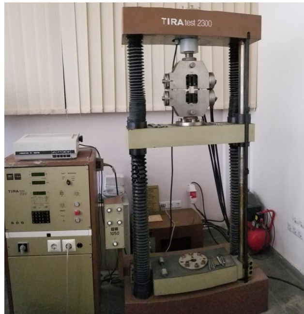
Fig. 3 - General view of the TIRA test 2300 breaking machine, Equipment manufacturer « VEB Werkstoffprüfmaschinen», Germany
