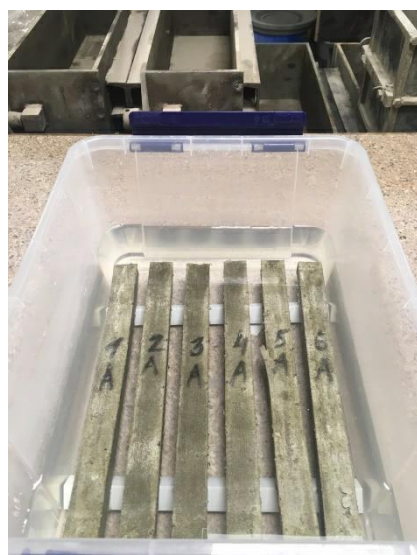
Figure 3. Samples of elastic two-component waterproofing "HydroLastic"
