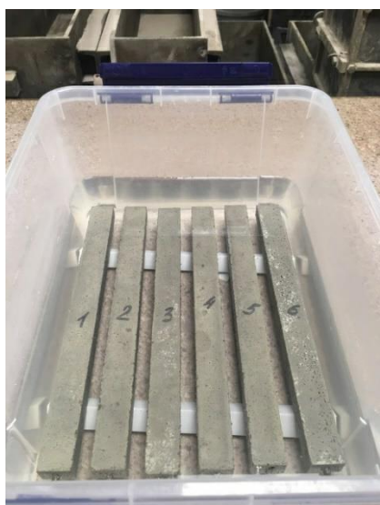
Figure 2. Samples of the repair composition "RM-W Plus"
