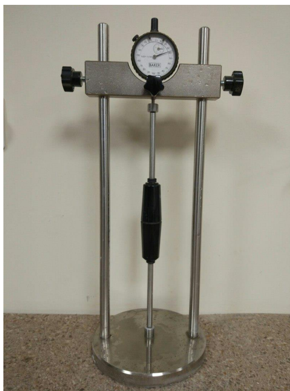
Figure 1. Device for measuring linear expansion
